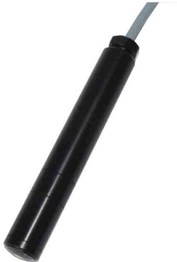
The OxyGuard Mini Probe is a membrane covered galvanic cell that generates an electrical signal proportional to the oxygen pressure it senses. It is a small version of the probe that has become the preferred choice of dissolved oxygen probe for fish farmers all over the world.
